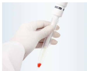
Pipettieren in enge Röhrchen
